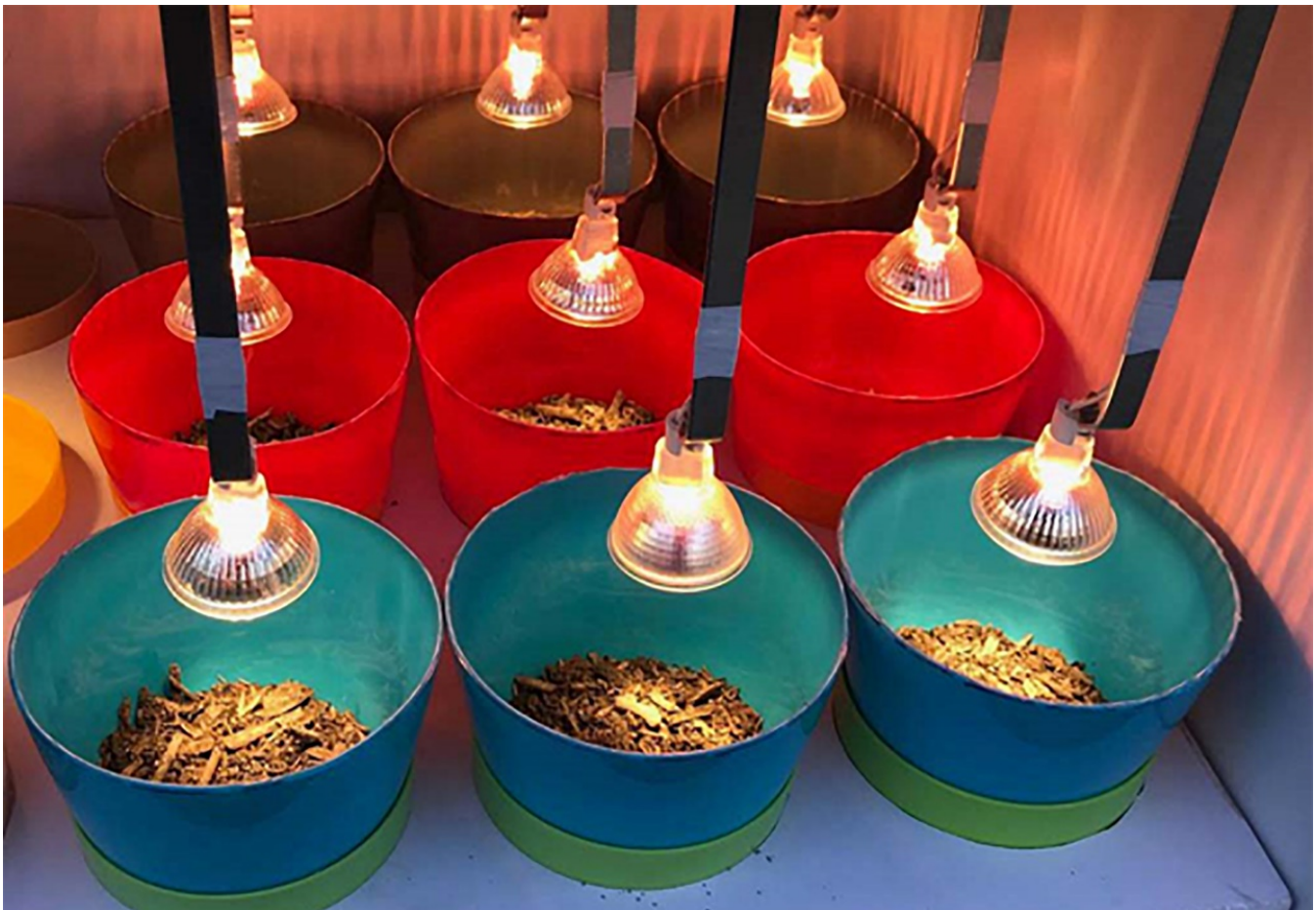
Figure 2. Extractor system for soil animals.
