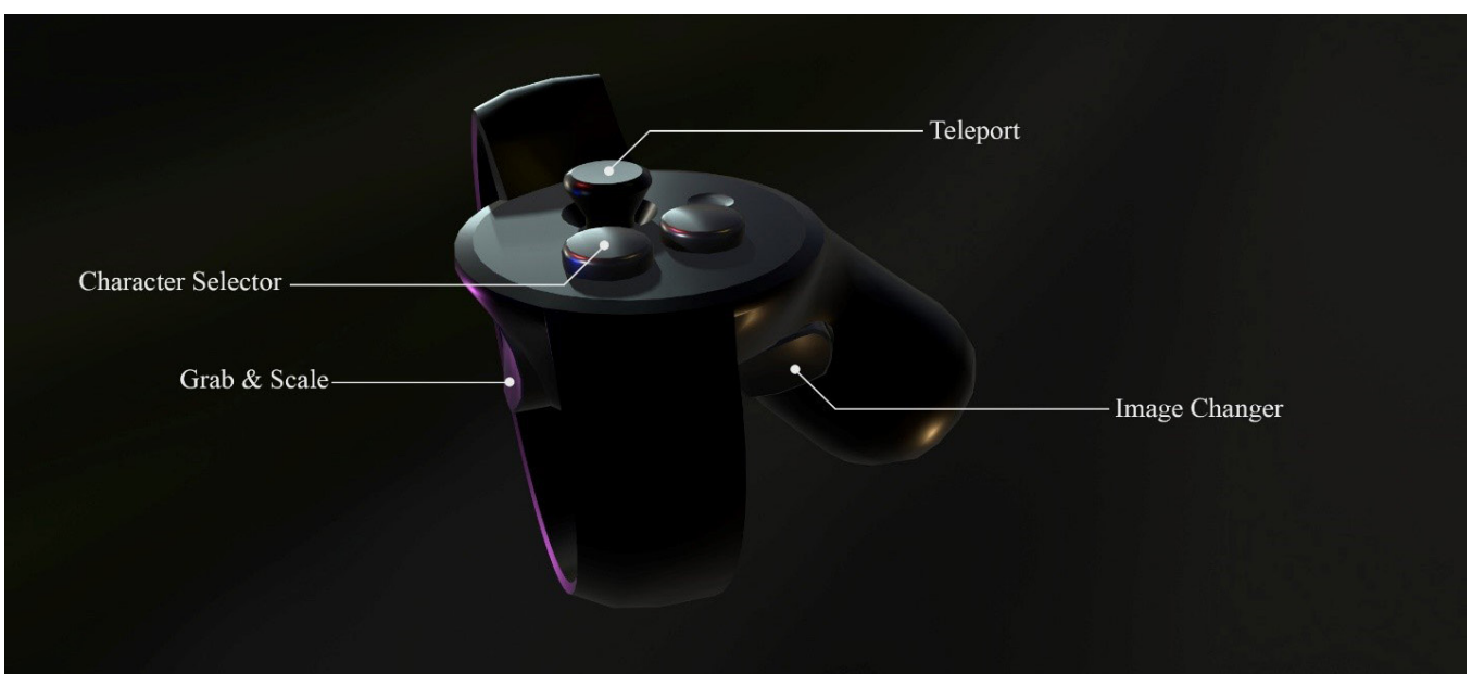
Figure 7. Illustration of the VR controller buttons with different functions (Oculus Touch Controller). https://zenodo.org/uploads/11081014 - suppl. 01
