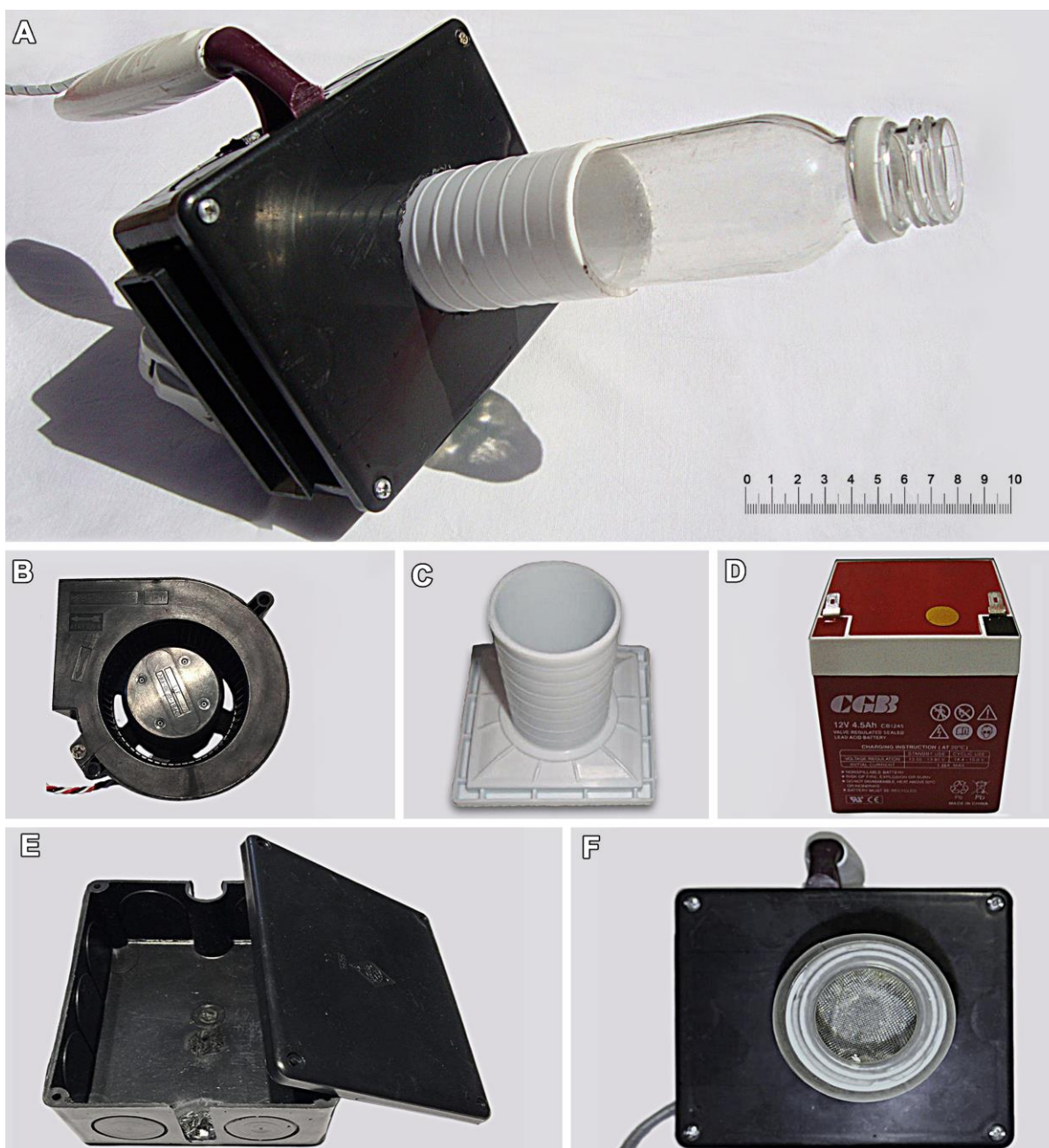
Figure 1. The ElePooter apparatus and its components: A. The complete system in lateral view; B. Centrifugal fan; C. Manifold; D. Chargeable battery; E. Main box; F. Frontal view of the device.
