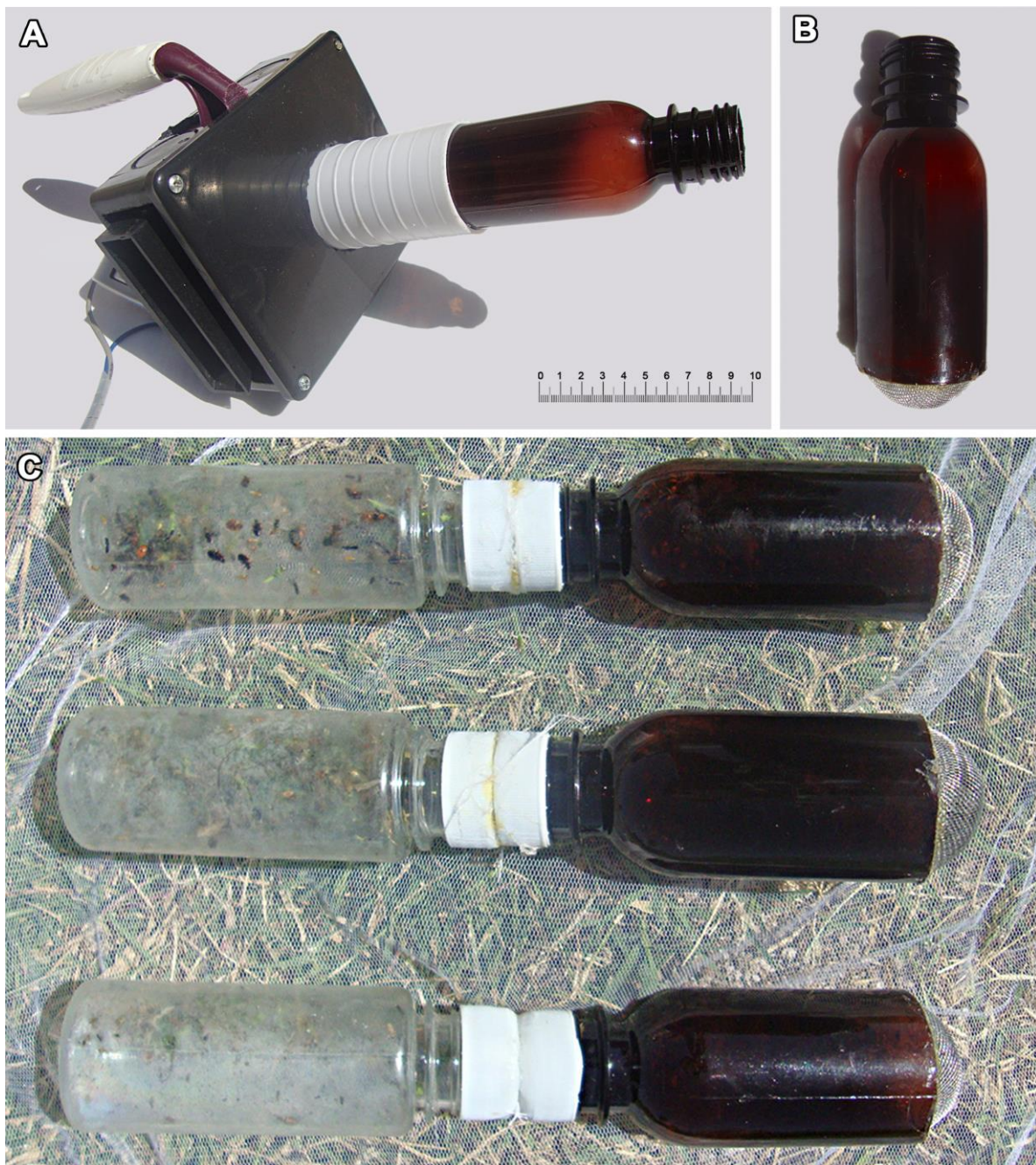
Figure 4. Specimens collected using the ElePooter with dark storage bottle: A. The complete system; B. Dark storage bottle; C. Coupled dark and transparent collecting bottles.
